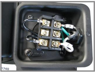
Figure 6. Drum motor wiring.
